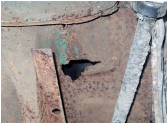
Front o/s inner wing near "A" post rot!
