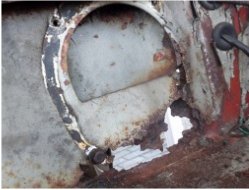
Corrosion right through both sides of plenum chamber
