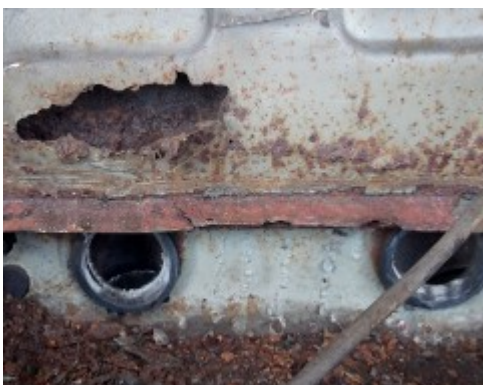
Bulkhead behind heater matrix rotten through
