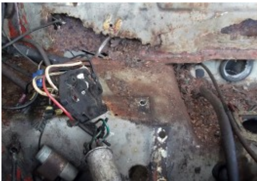
O/S plenum chamber rotted through the 2 walls
