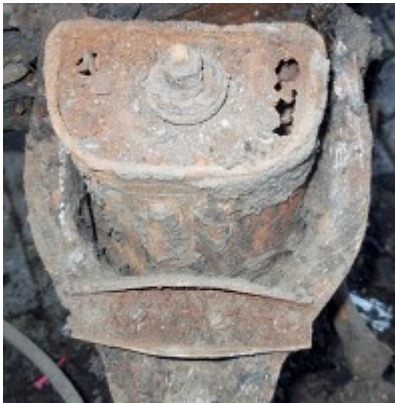
Rusted through front o/s suspension turret
