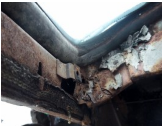
Corroded o/s "A" & Screen frame
