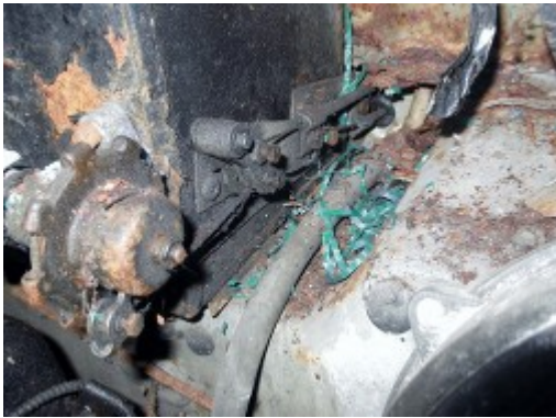
Heater cable setup & holed bulkhead
