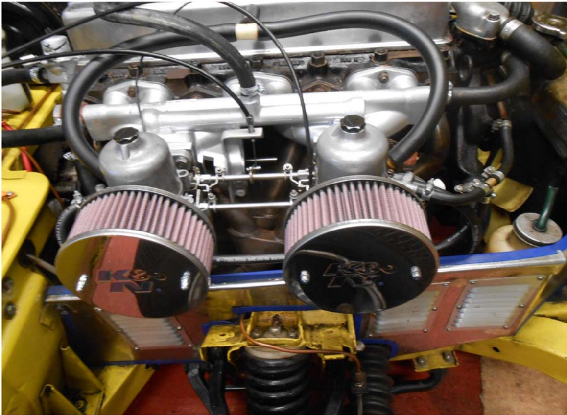
Picture 14 shows Carburetors and manifold throttle and choke cables connected along with new K & N Filters and petrol pipes.
