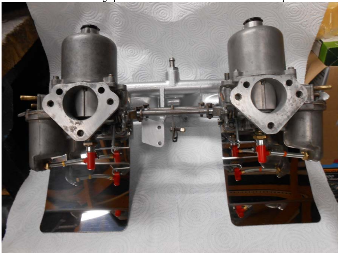
Picture 11 Carburetors fitted along with throttle and choke linkages
