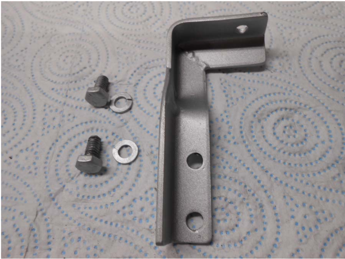
Picture 12 shows the adaptor bracket for the throttle linkage
