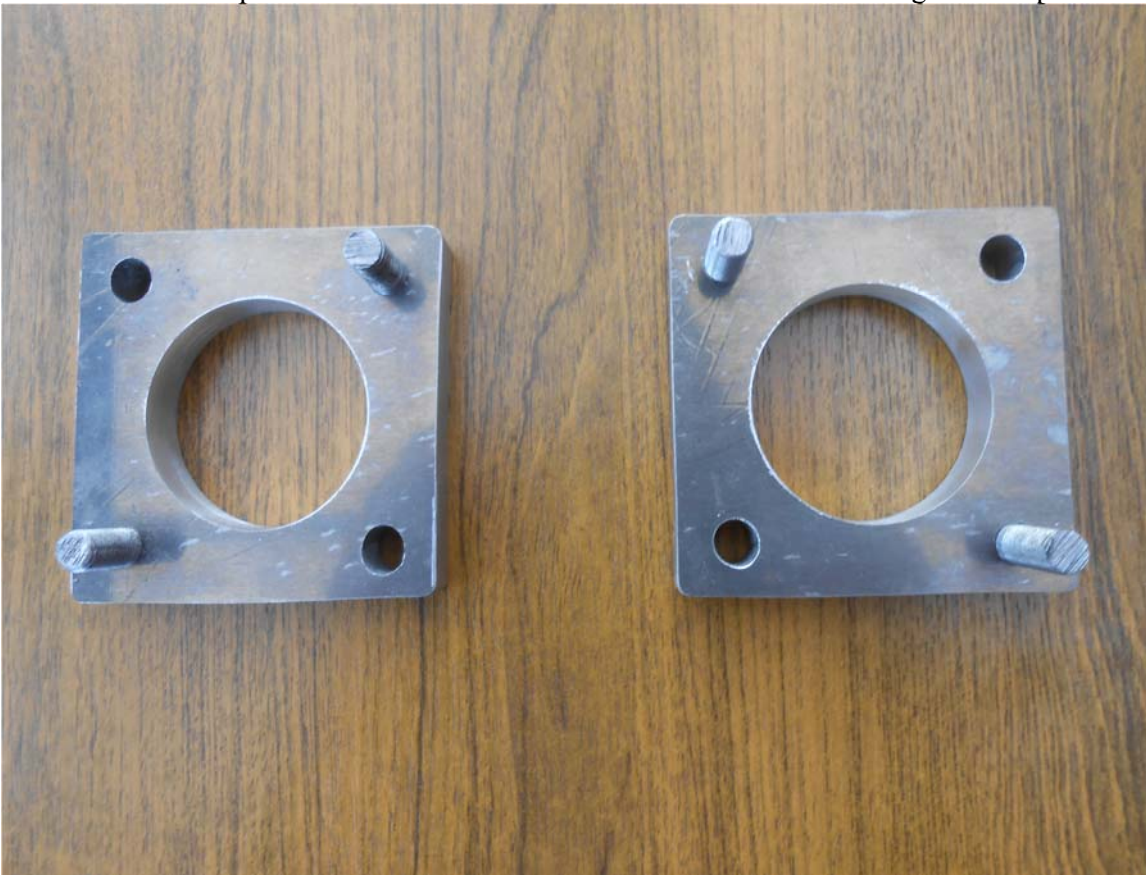
Picture 4 the aluminium adaptor blocks after drilling and tapping.
