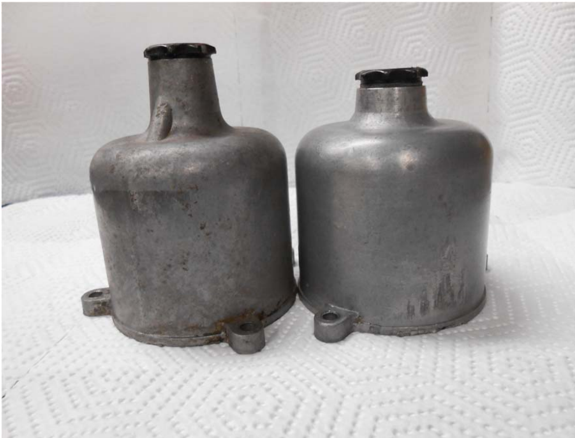
Picture 1 SU HS4 Dashpot on the left Dolomite Sprint SU HS6 Dashpot on the right
