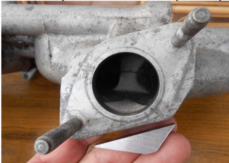
Picture 6 shows how much port needs to be opened up and aluminium piece to be welded
