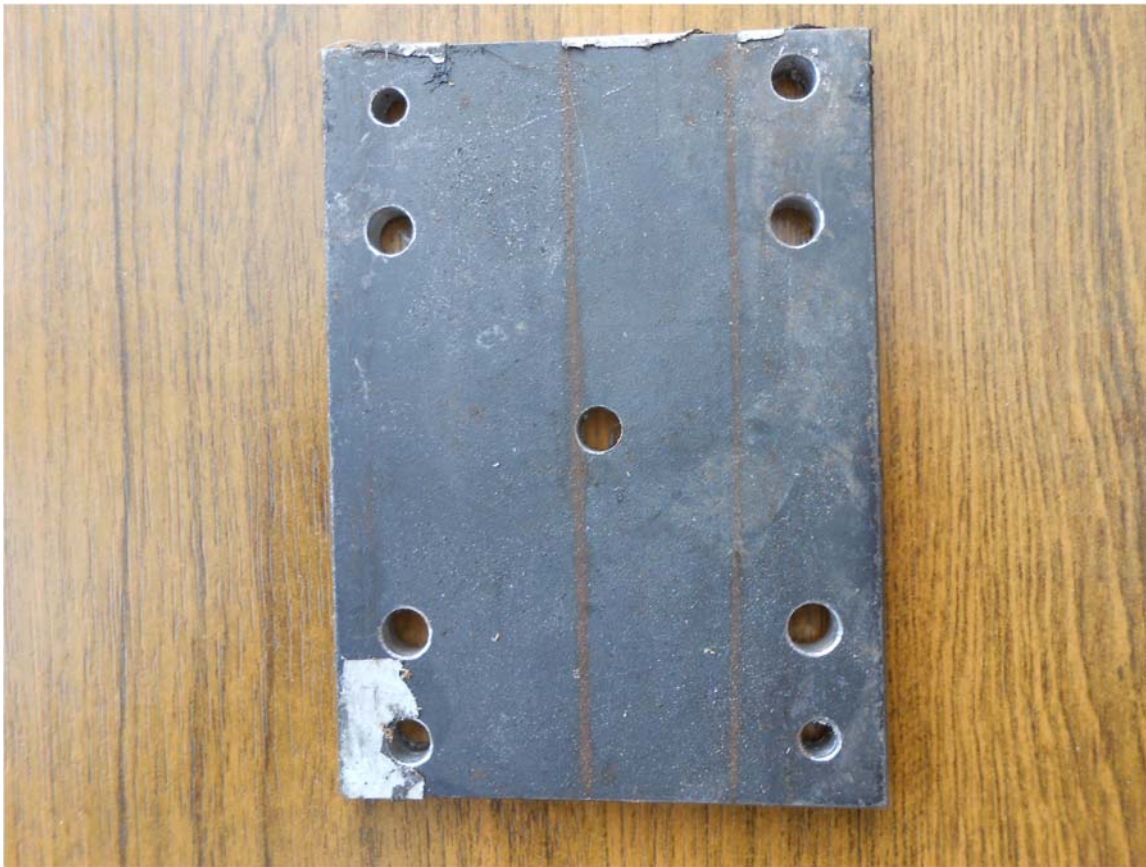
Picture 3 steel template which was fixed onto aluminium blocks for drilling holes in position
