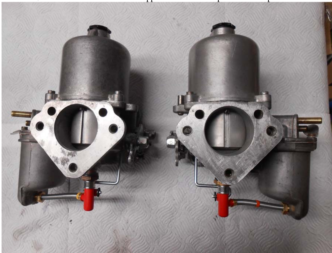
Picture 8 above shows both carburettors overhauled and ready to fit onto inlet manifold
