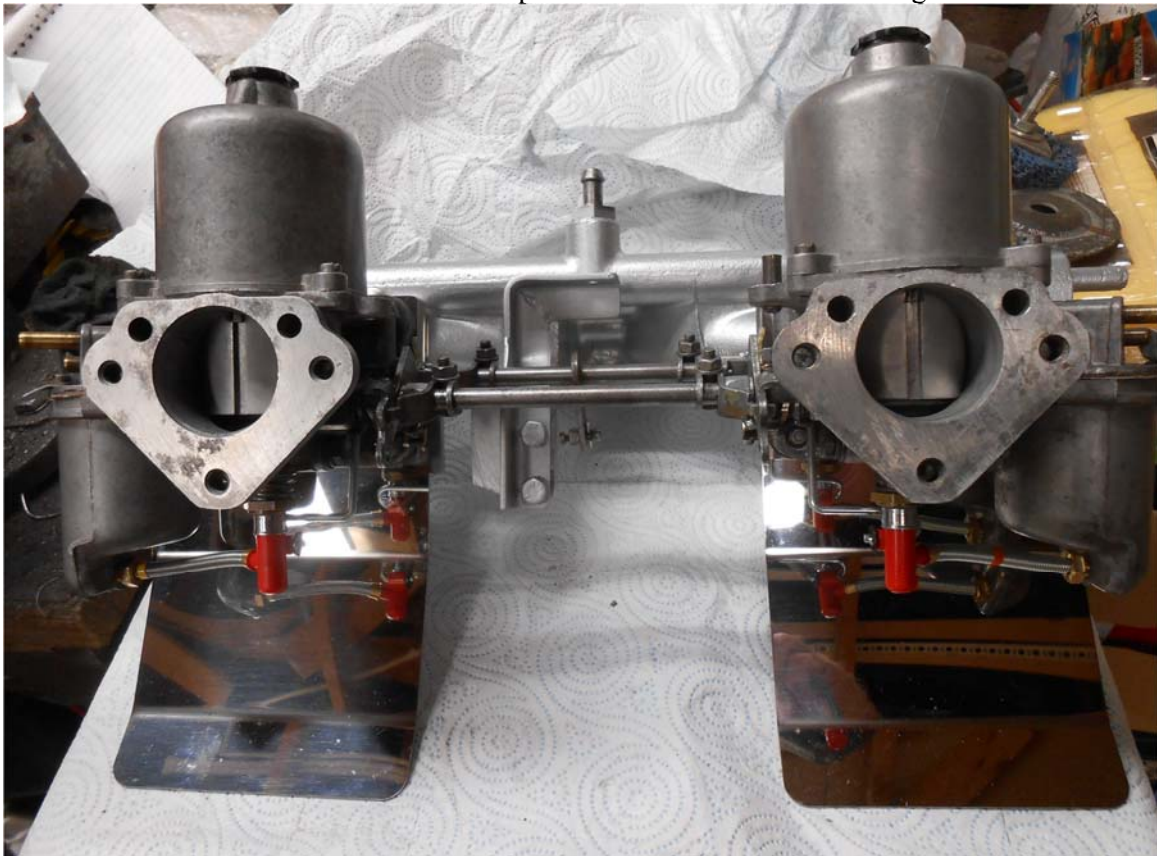
Picture 13 shows bracket and linkage set up with carburetors
