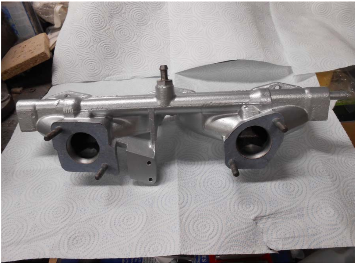
Picture 9 shows inlet manifold with ports opened up to inch and three quarters and gaskets made up and fitted.
